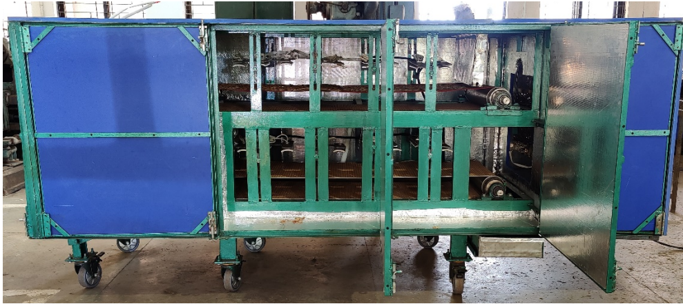
Fig. 2 Hot air-assisted continuous infrared dryer
