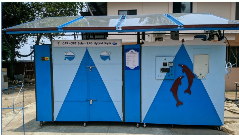
Solar-LPG hybrid dryer
