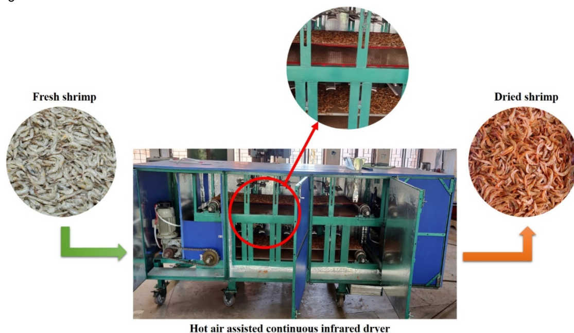
Fig. 3 Shrimp drying process in the hot air-assisted continuous infrared dryer
