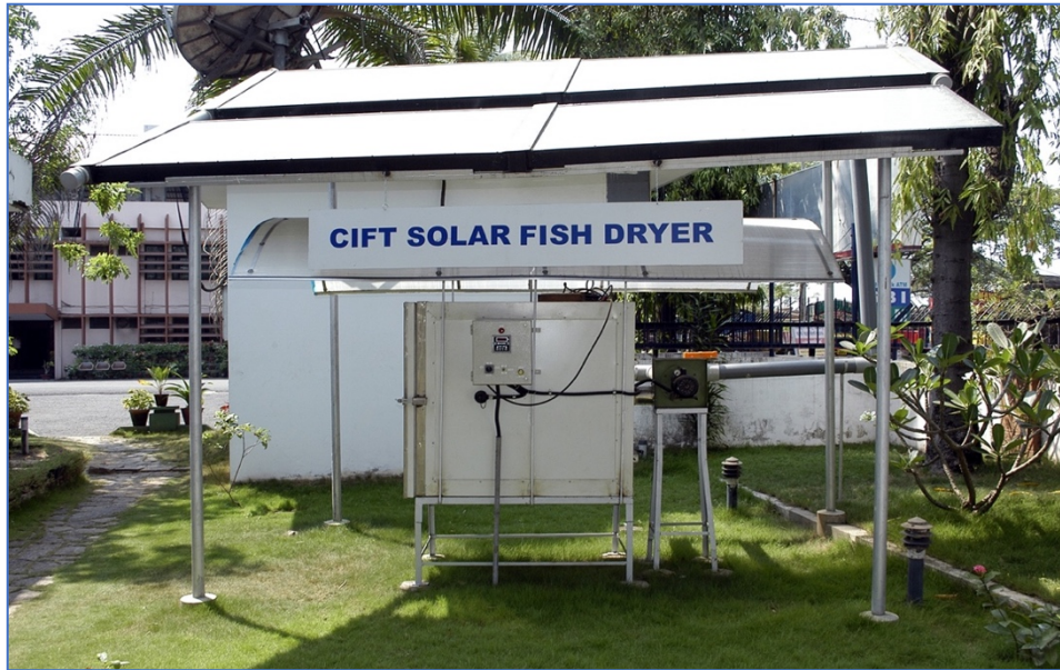
Solar-electrical hybrid dryer
