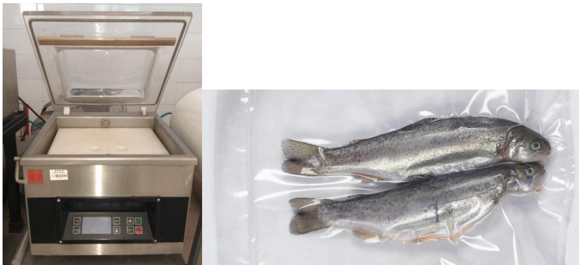
Fig. 1. Vacuum packaging machine and Vacuum-packed fish
