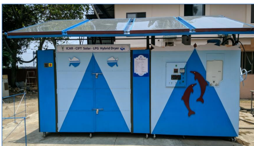
Fig. 2. ICAR-CIFT Solar-LPG hybrid dryer
