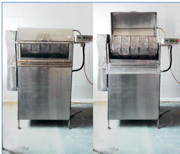
Fig. 7. Fish de-scaling machine with variable drum speed
