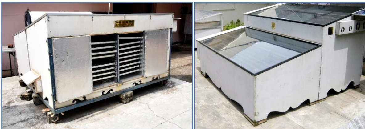
Fig. 4. ICAR-CIFT Solar-electrical hybrid dryer
