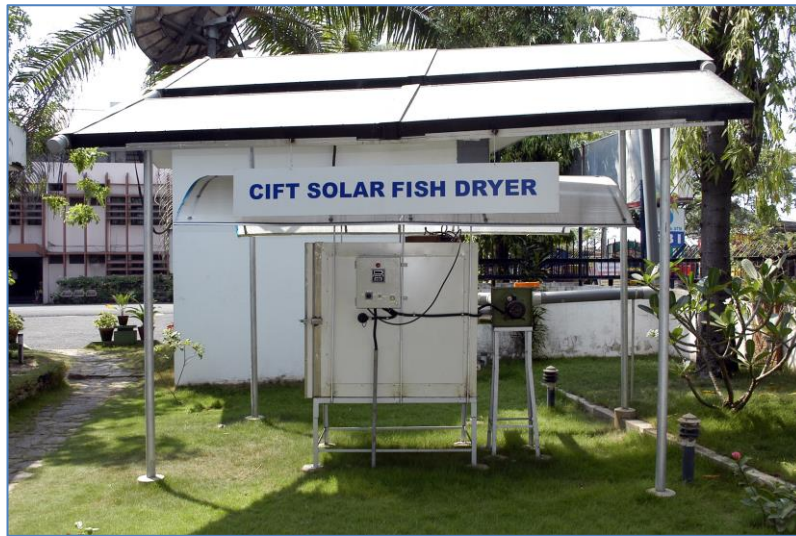
Fig. 3. ICAR-CIFT Solar-electrical hybrid dryer
