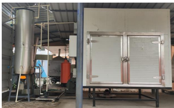
Fig. 1. Photograph of Solar-gasifier hybrid dryer developed at CIFT, Kochi
