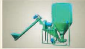
Feed Plant (Feed Mixer & Grinder)
