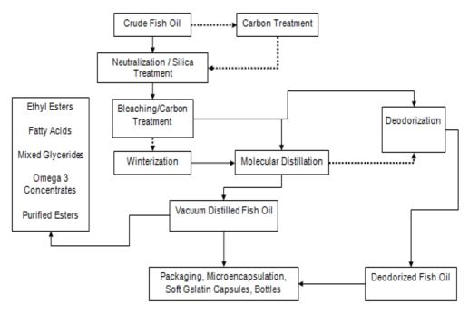
Process flow for Production of edible and pharmaceutical-grade fish oils and derivatives
