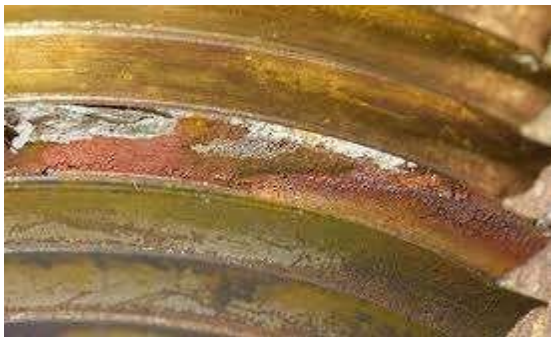
Corroded surface as a result of Selective Attack
