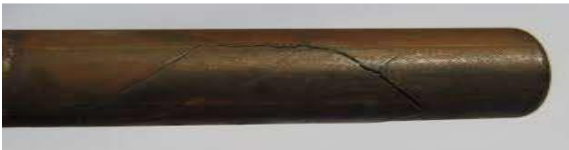
Cracking due to stress corrosion
