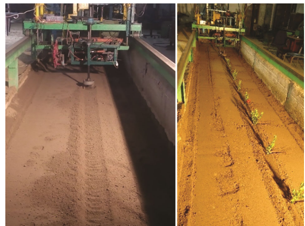
Fig. 9 — Soil bin laboratory evaluation of intra row prototype
