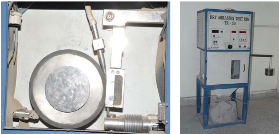
Figure 1. Rubber wheel /dry sand abrasion test apparatus
