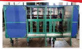
and gear arrangements, discharge chute and control panel. Drying experiments were conducted in this infrared dryer using various fishes and found that the drying time requirement was significantly less than that of conventional dryers.
