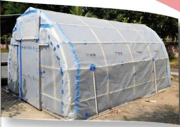
The tunnel dryer is made of UV stabilized transparent polythene sheet for roof cover, black
