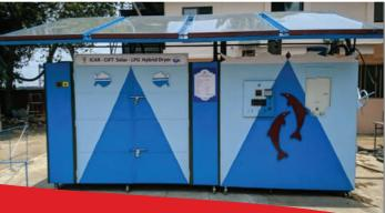
The dryer helps to dry fish using solar energy supported by environment friendly LPG based water heating source. In this dryer, fish could be dried using solar energy during sunny days, and when solar radiation is not sufficient especially during cloudy/ rainy days, LPG back up heating source will be automatically actuated to supplement the heat requirement.
