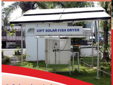
2. Solar-electrical hybrid dryer (40 kg)
