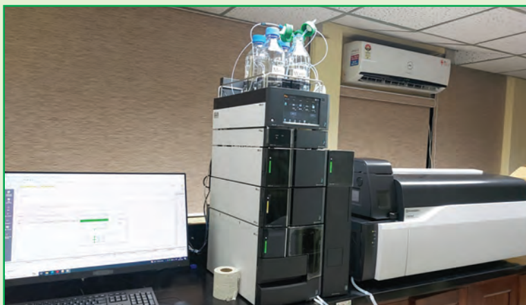
Newly installed and commissioned LC-MS/MS (LC-MS TQ-8045, Shimadzu)
