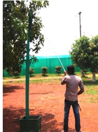
Modified mango harvester with transmission hose
