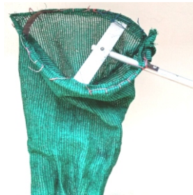
Modified mango harvester
