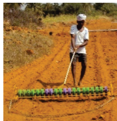
Manual drawn onion seeder with metal wheels
