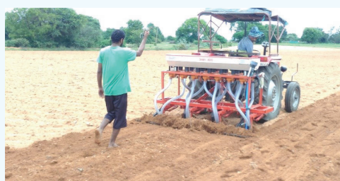
Seed cum fertilizer drill at work in Raguttahalli village: KVK, Chikkaballapur
