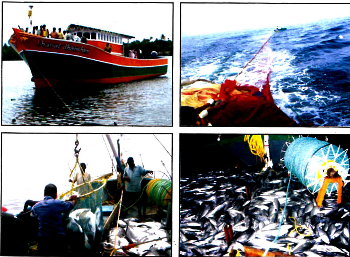
Fig. 10.5 A small-scale mechanised purse seiner, based at Cochin, India and views of setting, brailing and landed catch
