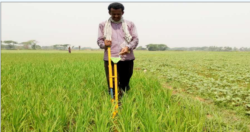
Injector type urea briquette applicator (top dressing)
