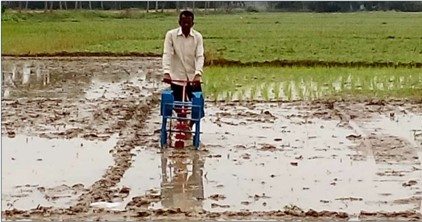
Two row urea briquette applicator (basal application)
