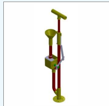
Non-continuous injector type urea briquette applicators made of polyvinyl chloride (PVC) pipe developed by IFDC
