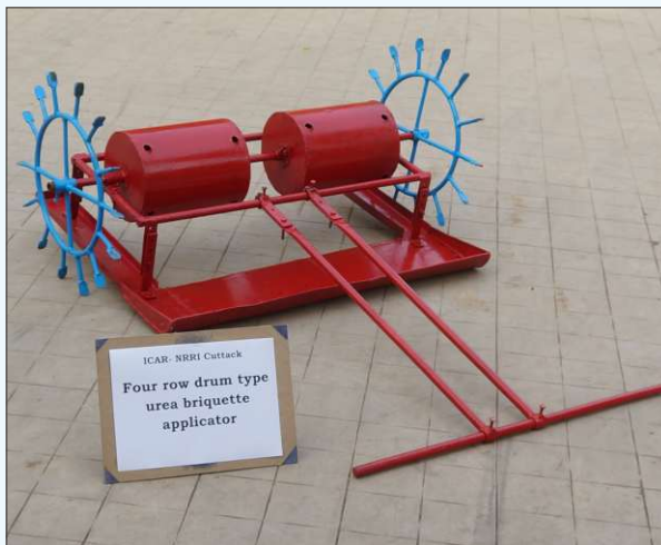
Plate 11. Manually pulled four row briquette applicator
