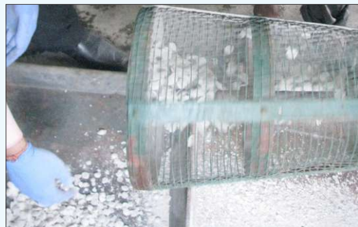
Plate 6 b) Preparation of urea briquettes in briquette making machine
