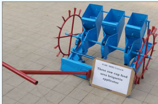
Plate 10. Manually pulled three row briquette applicator
