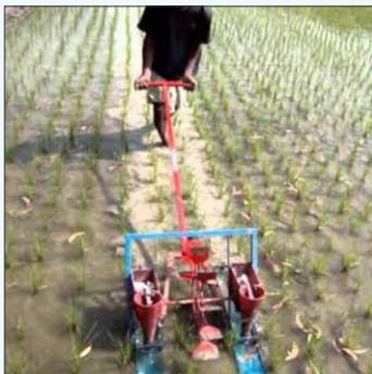
Manually operated push type continuous operation two-row USG applicator developed by Bangladesh Agricultural Research Institute (BARI)
