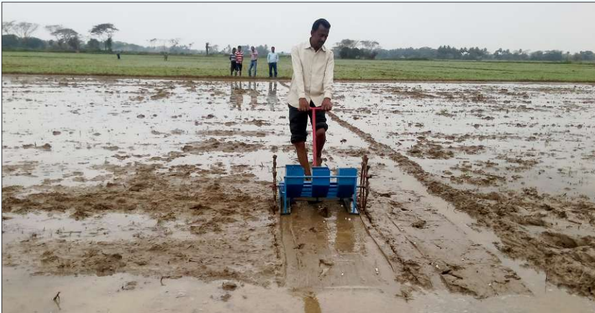
Three row urea briquette applicator (basal application)
