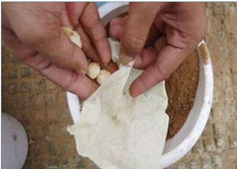
Plate 8. Buried bag technique to study urea hydrolysis
