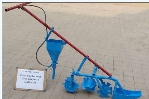
Plate 12. Urea briquette applicator mounted on conoweeder
