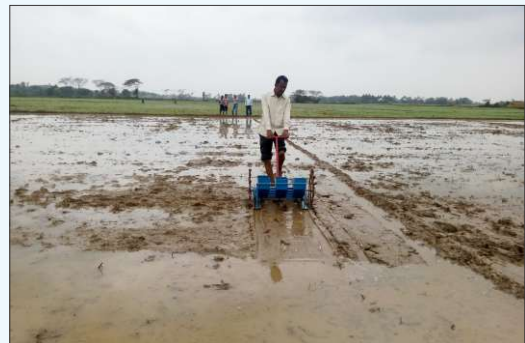
Plate 10. Manually pulled three row briquette applicator
