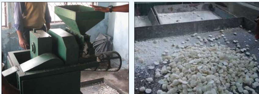
Plate 4. Urea briquettes/urea pellets prepared from granular urea in briquette/pellet making machine (breaking 25-30%)
