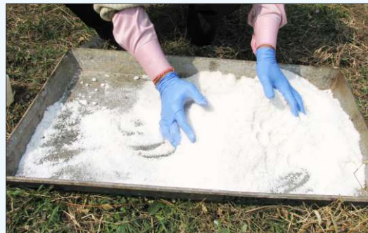
Plate 6 a) Addition and mixing of filler material and binder to prilled urea
