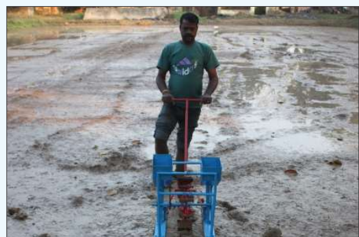
Plate 9. Manually pulled two row briquette applicator
