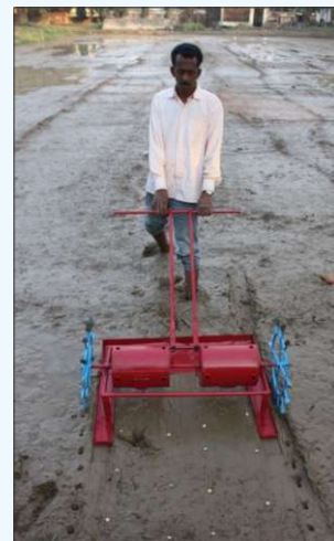
Plate 11. Manually pulled four row briquette applicator
