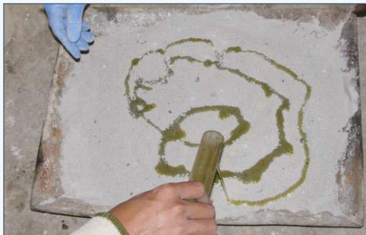
Plate 6 a) Addition and mixing of filler material and binder to prilled urea
