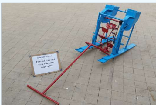
Plate 9. Manually pulled two row briquette applicator
