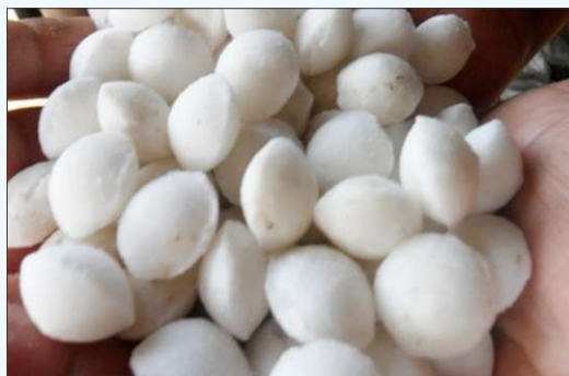
Plate 2. Oval shaped supergranules (urea pellets/briquettes) prepared by mechanical compaction using briquette/pellet making machine.
