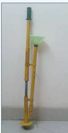
Plate 13. Injector type briquette applicator
