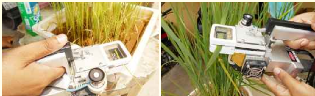
Fig. 2 Measurement of photosynthetic rate and stomatal conductance
