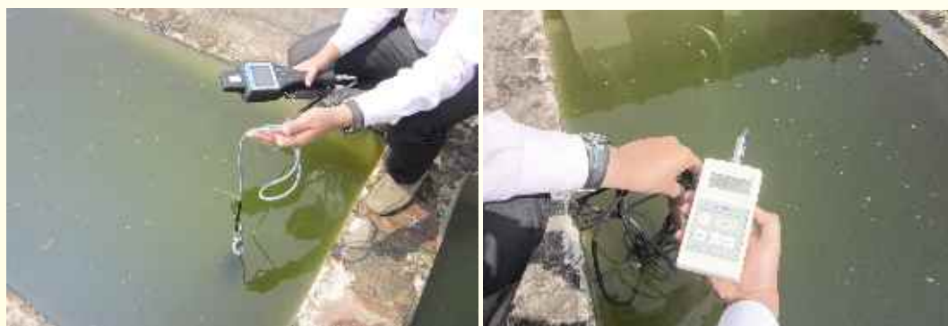
Fig. 1 Measurement of under water PAR and water quality parameters
