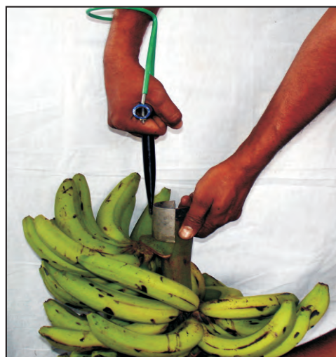
Fig 6: Banana comb cutter in operation
