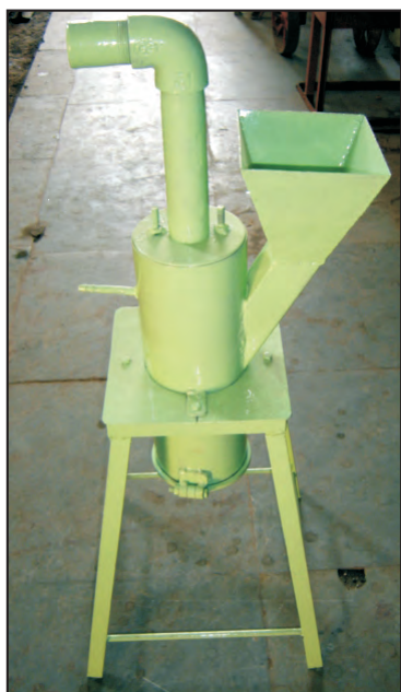
Fig 74 : Garlic Peeler developed by Udaipur Centre
