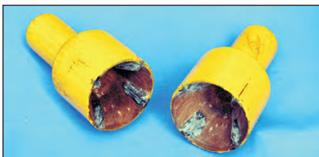
Fig 37: Hand held device to break pomegranate fruit
