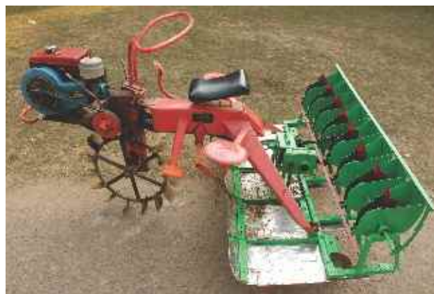
Fig. 2.10. Eight row self propelled paddy seeder with cup type seed metering mechanism
