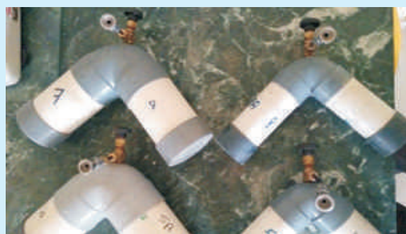
Canister developed for gas collection in goats
