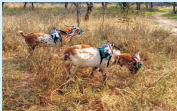
Figure 2: In vivo methane estimation using SF 6 technique
