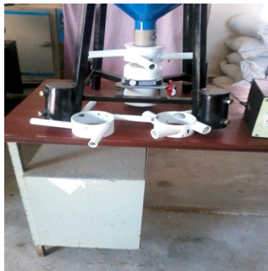
Fig. 4. Distribution system with four pipes
