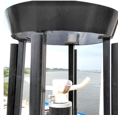
Fig. 5. Distribution system with three pipes
