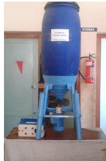
Fig. 2. Indigenously designed automatic feeder
