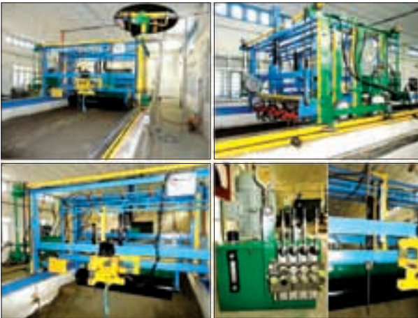
Automated soil-processing trolley and cone penetrometer
