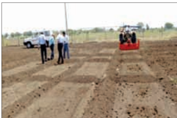
Tractor-operated check-basin former
