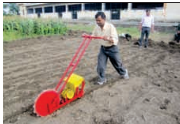
Manually operated multi-millet planter
