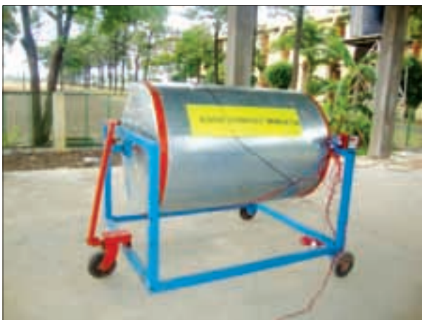
Rotating drum-type bioreactor
