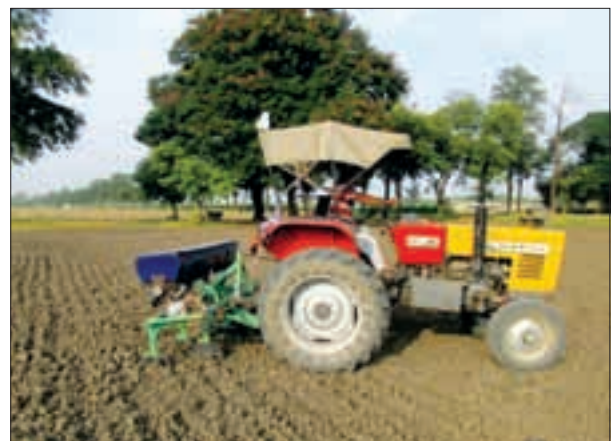
GPS-based variable rate fertilizer applicator
