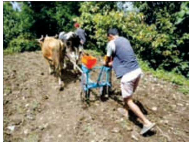
Two row zero-till seed drill
