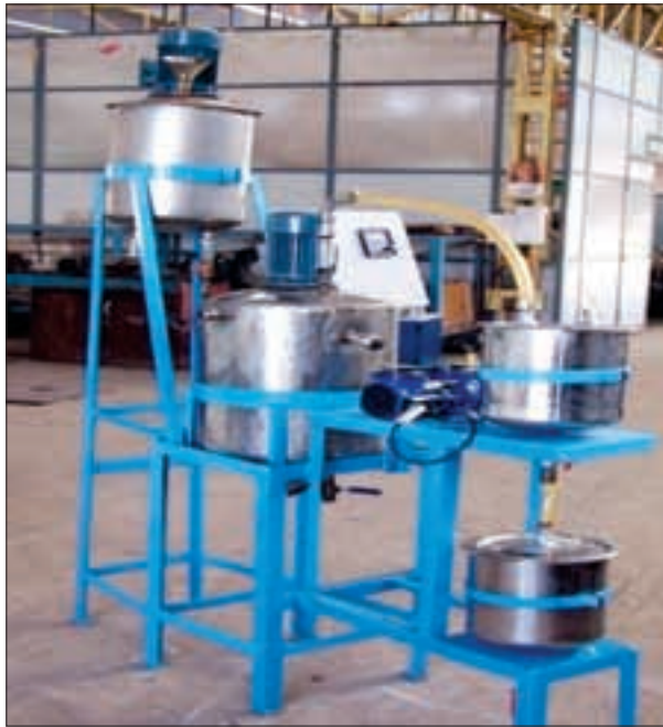
Plant for glycerol refinement
